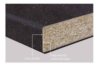
Our **postformed worktops** have a unique, advanced, high density protective layer underneath the laminate edge that makes the edge of the worktop more resistant to impact and stops any show-through of the chipboard core.
